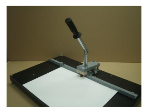
The die is mounted on the top press plate of the MP-1 press, so the cutting position is fixed relative to the table top. This allows the rectangular sheet to be aligned to one side and corner.
