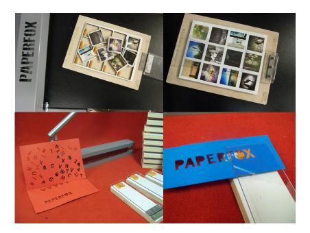
In this case, the positioning is done to the marks on the transparent folding plate connected to the die by a hinge. The die cutting can be done on the fold-out plate or you can use an other cutting plate after folding out the transparent positioning plate.
