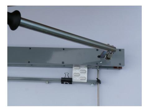
The KB-32 creasing guide bar can also be made suitable for positioning at die cutting with a simple trick using a paper clip.
