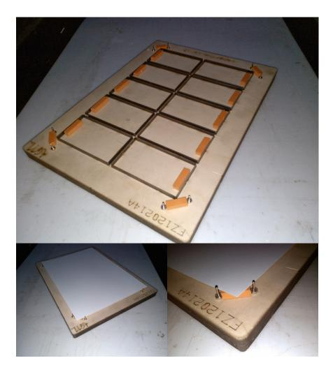
With special spring positioning pins, the inaccuracy caused by sticking guides on the ejector rubber can be reduced. Typically, eight pins placed near the corners can position the sheet stably. The spring pins can be pushed down during the die cutting process.
