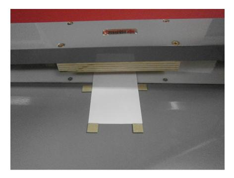
Stick double-sided adhesive tape to a thick cardboard sheet. Cut out the positioning elements and stick them to the appropriate positions on the workbench of the diecutting machine.
