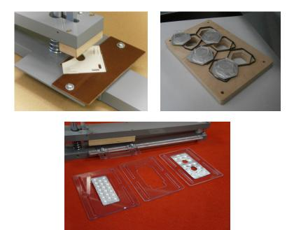
Complex shaped objects may not always be positioned to some points. When die cutting blisters or shaped objects, the function of the positioning elements is also to fix the object and secure it against movement. In this case, the exact location of the die cutting can be ensured by means of a counter-shaped guides.
