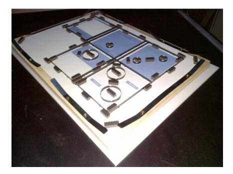
If you can't get special positioning pins, you can also solve the problem with folded spring steel strips.
