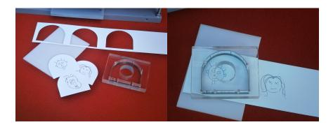
Die cutting tools made of transparent material (for example polycarbonate) can be placed on the sheets to be punched while the printed pattern is visible. These tools usually have no ejector rubber because it would cover the pattern. In this case, the workpiece can be pushed out of the tool through a hole in the die. This positioning mode is primarily recommended for flat punch machines.
