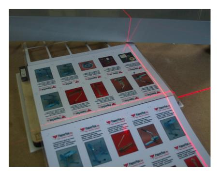
The alignment marks on the printed sheet or the characteristic points of the print can be aligned with the laser "+" mark. The method is not very accurate and a bit cumbersome.
