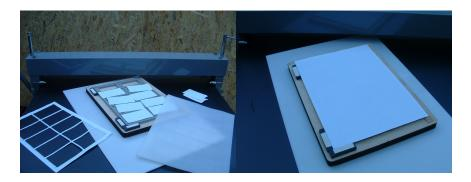
On cylinder die cutting machines, the positioning to the machine table is not applicable, so the positioning elements should be fixed on the die cutting tool. This procedure can also be used for flat die cutters. The easiest way is to make the positioning elements of thick cardboard and doublesided self-adhesive tape and stick it on the ejecting rubber of the die. At least three positioning elements are required, but even more can be used for a more secure registration.
