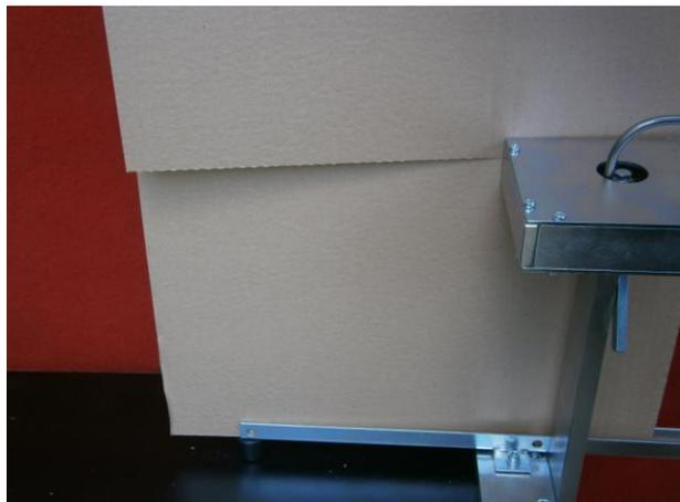
Select the cutting tool, set the desired cutting position and push a sheet through the Box Maker as in the picture.
