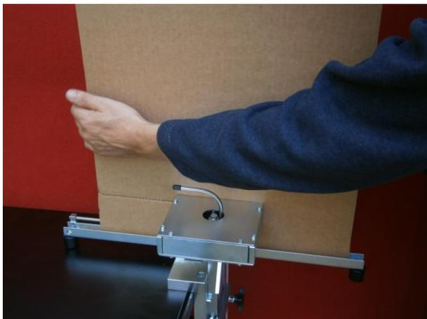
Select the perforating tool, set the perforation position (E) and perforate all the 4 side of the sheet.
