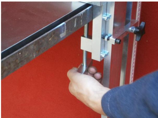
You can fix the Box Maker on a table which is strong enough to hold the device during operation.
