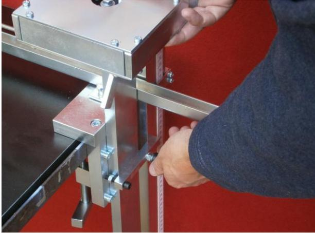
Hold the knife covering box and loose the scale fixing screw. Now you can move the steel frame up and down. Select the desired position with the help of the scale and fix the scale fixing screw.
