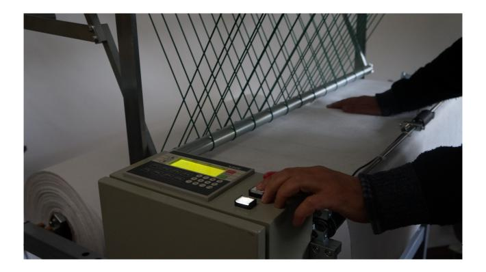
By continuously pressing the motor start button, the roll material can be inserted in to the unwinding unit. The insertion in to the unwinding unit usually also requires manual assistance. After unwinding some material, then the rewinding continues even after the start button is released.
