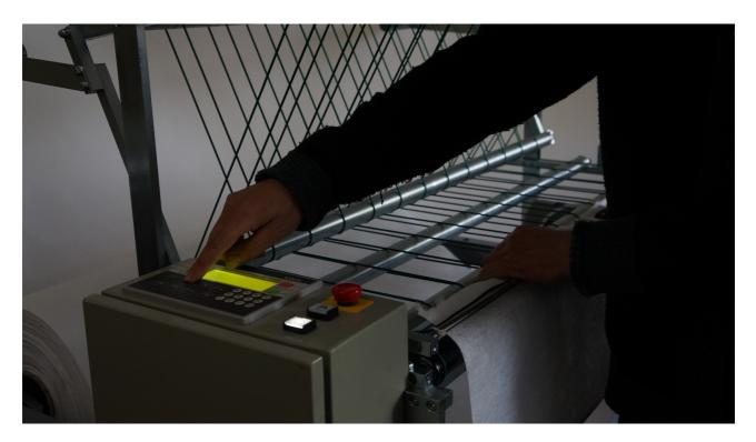
Raise the feed roller equipped with a length gauge and pass the rewinding material under it. When the edge of the material to be wound is in the line of the rail that helps cutting, reset the length gauge by pressing the F2 key. (The roll counter can also be reset with the F1 key)
