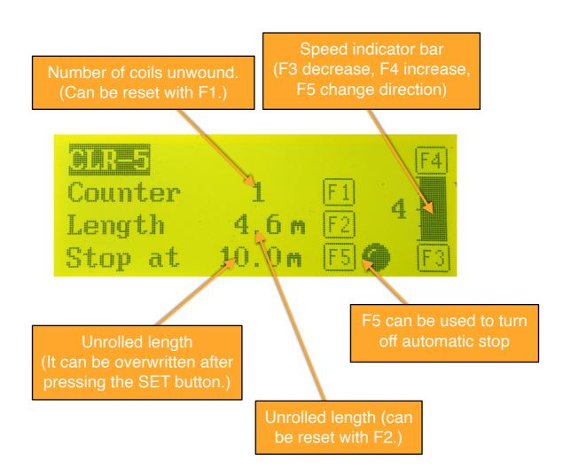
The speed of the conveyor belt can be adjusted in 4 steps with the F3 and F4 keys.
