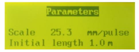
In the "Initial length" variable, is the length until you have to push the motor start button continuously to achieve the the continuous motor movement.
