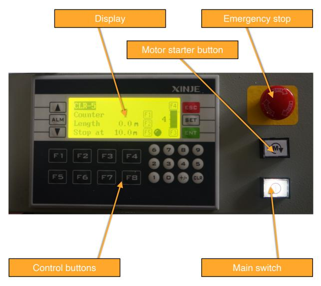
The device can be switched on by pressing the main switch. If the indicator light does not light up, check the condition of the emergency stop button. The emergency stop button can be reset to its default state by turning the red head.
