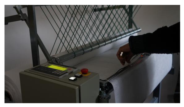
If the material is difficult to cut, you can use scissors, v. circular cutter as well.
