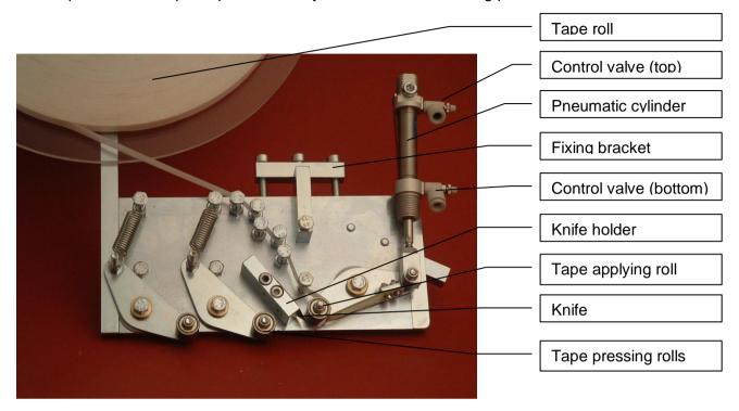
The TD-1 tape dispenser normally have only the accessories in the picture above. You can control the device with switching compressed air to the pneumatic cylinder. The device can be fixed with the fixing bracket to two 15x15mm rectangular steel bars.
