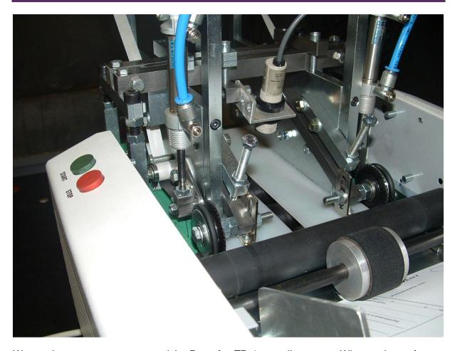
We used an optosensor to control the Paperfox TD-1 tape dispensers. When a sheet of paper arrives under the Paperfox TD-1 tape dispenser, the optosensor switches on the electric valve, and if the paper leaves the Paperfox TD-1 tape dispenser the switches off the valve. Then the Paperfox TD-1 tape dispenser cuts the tape.
