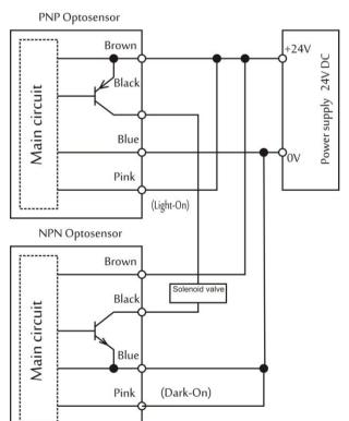
You can use two optosensors to controll your TD-1. When the paper reaches the PNP optosensor it switches on. The NPN optosensor is connected to be dark-on so it is also on. The pneumatic valve opens. As the paper reaches the NPN optosensor it switches off so the pneumatic valve switches off.
