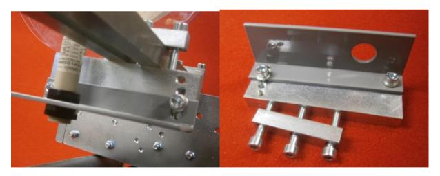
We use this mounting bracket in our HH-1 return receipt making machine. If you want to lay the tape band from the side to the oposit side of the sheet, then it is enough to use one optosensor to control the unit. The optosensor opens the pneumatic valve at the first side of the paper and closes at the end. fine adjustmens can be done by the adjustable flow control valves.
