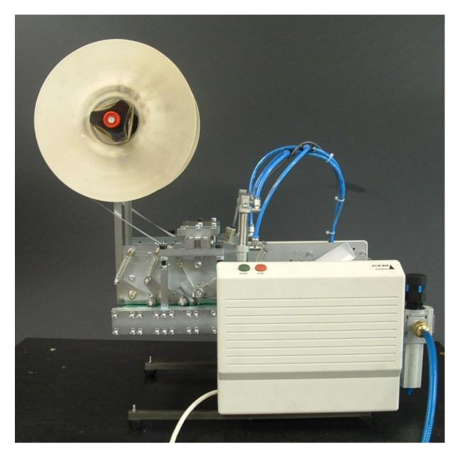
The Paperfox TD-1 tape dispensers were fixed with the fixing brackets onto two parallel 15x15mm steel bar. A conveyor belt runs under the Paperfox TD-1 tape dispensers and it is supported with rollers under the rollers of the Paperfox TD-1 tape dispenser.
