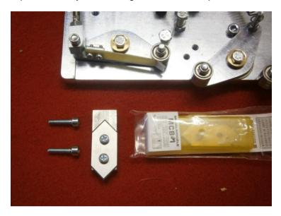
Remove the knife holder from the Paperfox TD-1 tape dispenser and you can remove the knife. Booth cutting edge of the knife can be used.
