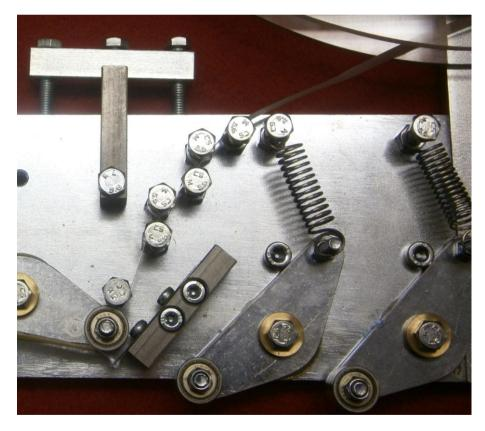
In the newest models we have inserted an additional screw to the TD-1 to ensure the proper guiding of the tape even if the paper don't runs properly under the TD-1.
