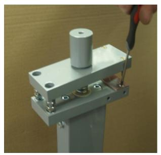
The VMP-1 cutting plate fixed with two screws into the MP-1 paper punch. You can replace the cutting plate after removing these screws. You can use booth side of the VMP-1 cutting plate.
