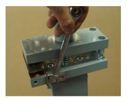
Mount the back paper stops with two M6x10 screws and washers on the paper punch. Use a 10mm wrench to fix the screws.
