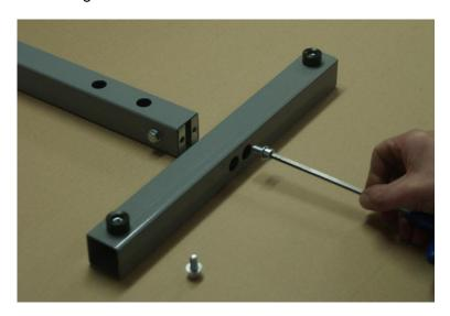
**2.** Assemble the vertical component of the frame with 2 pcs M8 imbus screws and washers. Use a 6mm hexagon tool.
