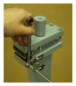
Mount the side paper stop on the paper punch. Use the M6 washer. Fix it with 10mm wrench. (You can mount the side paper stop to any side of the paper punch)
