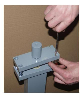
The tool (usually EP-1 euro slot tool) can be changed after removing the 2 pcs 3,5x35mm screws.
