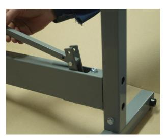
**4.** Insert the second screw into the pedal and fix it in the right position.
