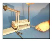
Release the female screw of the M8 setting screws at the back of the machine, set the parallelism and fix the screw again.
