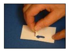
After longer usage or especially after changing the tool maybe that the machine don't cuts in the same way the whole shape which you want to cut. A part of the shape was cut well, but the other side not. In this case the setting of the parallelism of the machine can help.
