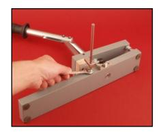
Mount the side paper stop on the paper punch. Use the M6 washer. Fix it with 10mm wrench. (You can mount the side paper stop to any side of the paper punch)
