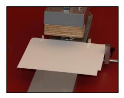
Set the position of the paper stops so that when you set the side of the sheet to this paper stops the paper punch should punch the hole in the proper position. For special tasks you can use special paper stops.
