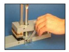
Mount the back paper stops with two M6x10 screws and washers on the paper punch. Use a 10mm wrench to fix the screws.
