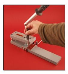
The VMP-1 cutting plate fixed with two screws into the MP-1 paper punch. You can replace the cutting plate after removing these screws. You can use booth side of the VMP-1 cutting plate.
