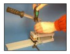
The tool (usually EP-1 euro slot tool) can be changed after removing the 2 pcs 3,5x35mm screws.
