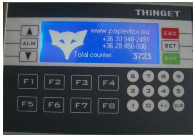
In the next screen you can find our contact dates and the total counter. This counter can't be reseted and sows the total number of perforation which the machine has made.
