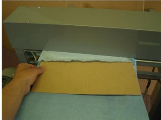
Guide the paper under the perforating tool. You can use for this purpose a sheet of card or corrugated paper as in the picture.
