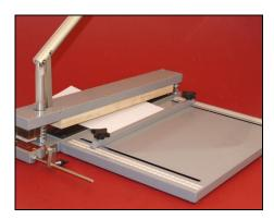
You can mount the MA-500 table to the Paperfox KB-32 multifunction press with two M6 screws.
