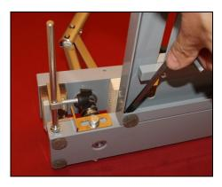
After changing the toll is it possible that the position on the scale don't indicates accurately the position of the crease on the paper. In this case you can remove the mark on the paper guide of the MA-500 table with petrol and you can make a new mark in the proper position with an alcohol marker pen.
