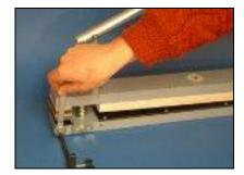
You can mount the guide for creasing (1) with the two bars (2).
