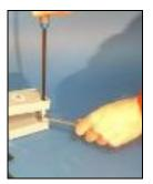
Release the female screw of the M8 setting screws at the back of the machine, set the parallelism and fix the screw again.
