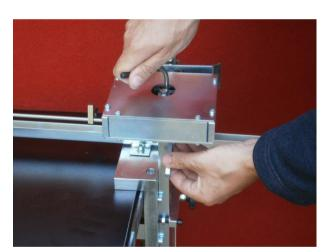
The Box Maker has a revolver head with a perforating and a cutting knife. You can select the desired tool with loosing the tool fixing arm and turning the tool changing arm into the proper position.
