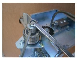
Not all corrugated paper is the same, so you sometimes have to set the depth of the perforation so that the box could be folded easily, but the corrugated paper won't break when folding.
