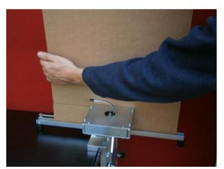
Select the perforating tool, set the desired perforation position and push a sheet through the Box Maker as in the picture.
