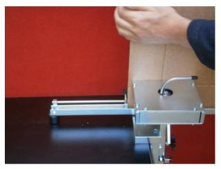
Select the cutting tool, set the position of cutting and set the paper stop so that it should limit the cutting length to the desired size.
