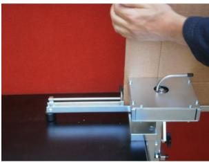
Select the cutting tool, and set the cutting depth with the paper stop. The cutting position is the same as the perforation position so you don't need to set this position again.
