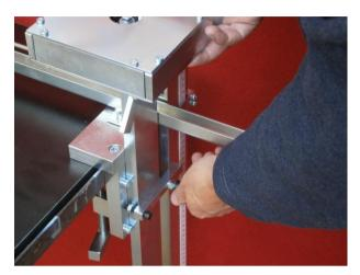
Hold the knife covering box and loose the scale fixing screw. Now you can move the steel frame up and down. Select the desired position with the help of the scale and fix the scale fixing screw.
