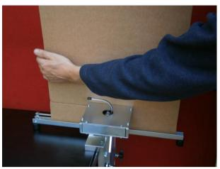
Select the perforating tool, set the perforation position (E) and perforate all the 4 side of the sheet.
