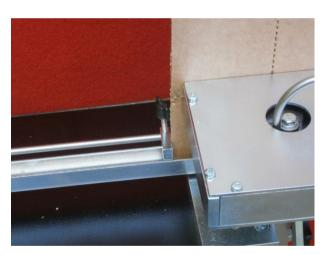
If you want to cut or perforate the sheet not in the whole width, you can set the paper stop into the proper position to limit the cutting/perforating length. Loose the M5 manual screw and set the paper stop into the proper position. Fix the M5 screw again.
