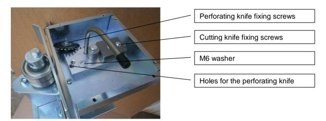
The perforating knife has a long life time, so presumably it doesn't have to be replaced. There are two threaded holes for this knife. If you can't set the proper perforating depth with the eccentric shaft of the paper supporting bearings, then you can screw the fixing screw of the perforating knife to the other threaded hole. Do not forget to put the M6 washer under the perforating round knife.
