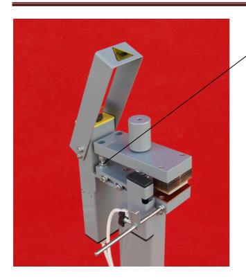
You can set the parallelizm of the MPE-2 with this two screws. You can set the M8 screws with a 6mm hexagon tool, and you can fix it with fastening the nut with a 13mm wrench.
