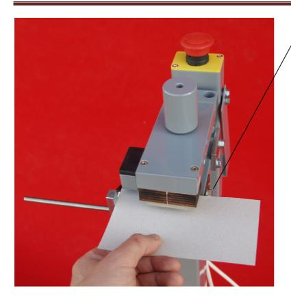
Back positioning paper guide at the other side of MPE-2. You can set the distance of punchings from the back edge of paper with this guide. You can set similar guide to the other side of MPE-2 too, if you remove the automatic start switch and use a foot switch. (extra acessory)
