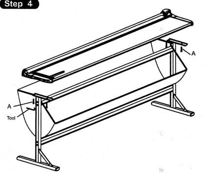
X Note: Not to fully tighten the screws before well assembling the trimmer onto the stand.
